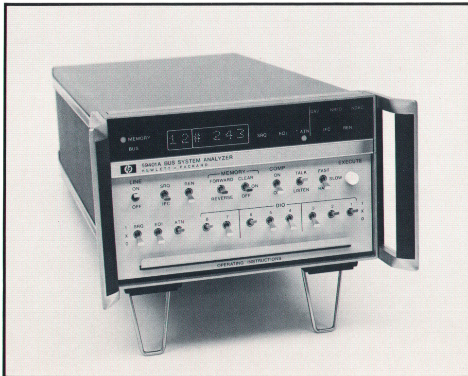
Fig. 1. Model 59401A Bus System Analyzer monitors activity on the HP Interface Bus, displaying the instantaneous status of all bus signal lines. It can also be a bus controller using programs stored in its memory or program steps set up on the front-panel switch register.
